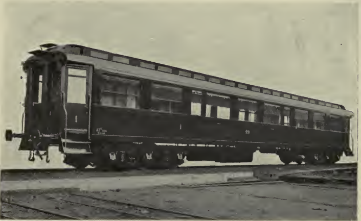
TWELVE-WHEEL BOGIE CARRIAGE (P.O.).
